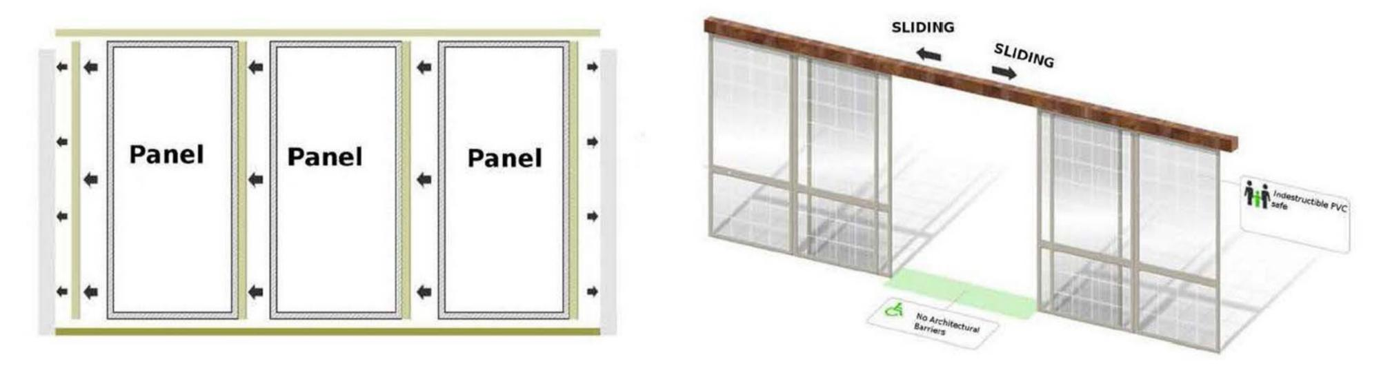
Litra USA retractable roofs is possible with two solutions of roofs: Standard Retractable Roofs or Sunroom Roofs. They can be fixed (fixed enclosures) or sliding (sliding roofs systems). The structure is completely removable and it's regarded by municipalities as a non permanent structure.
